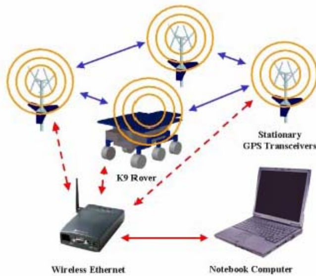
Figure 5 –SCPA architecture - A localised GPS system
