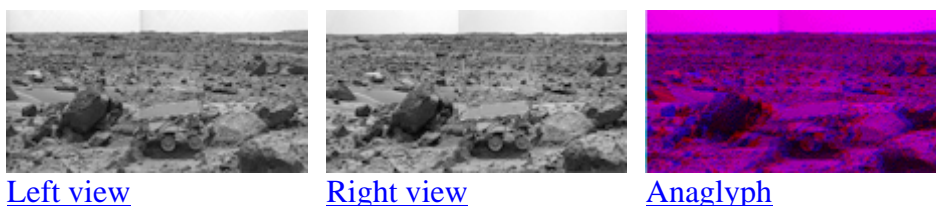
Figure 3 – The left and the right views from NAVCAM combined to give a 3D image.
